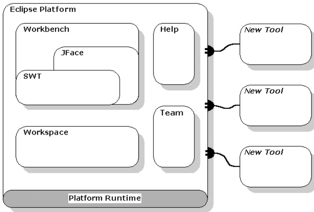
Figure 2. Eclipse Platform architecture.
