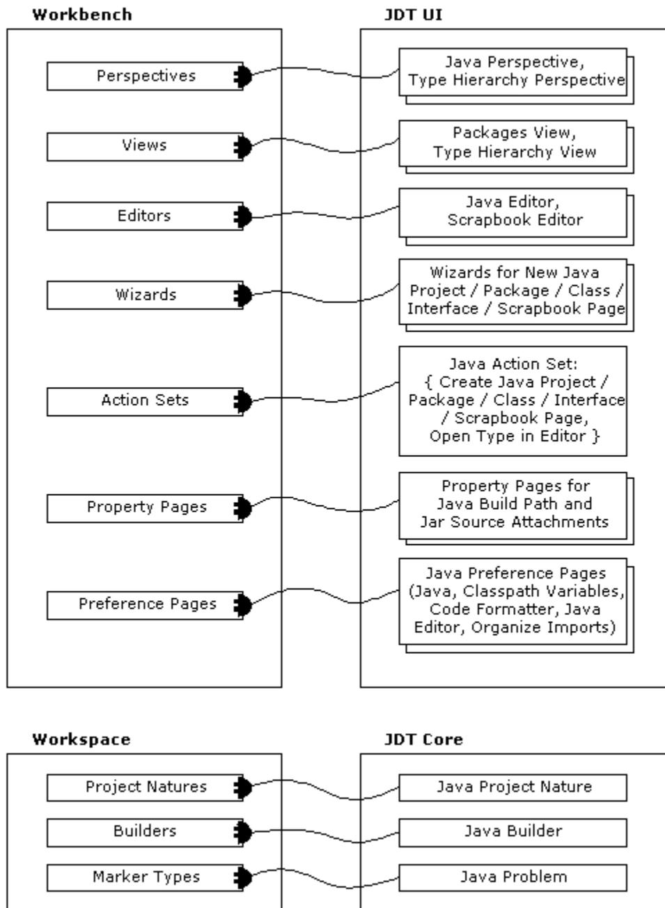
Figure 4. Key connections between JDT and Eclipse Platform.
